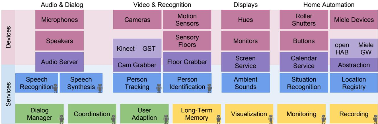
**Fig. 3** Functional system overview. Vertical *stacks* describe functional areas of the architecture. Abstraction layers are depicted horizontally. Hardware is colored in lavender, sensor/actuator abstraction in purple, and functional components (partially available at the robot) in blue. Behavioral components (green) and cross-cutting concerns (yellow) are related to many stacks.
