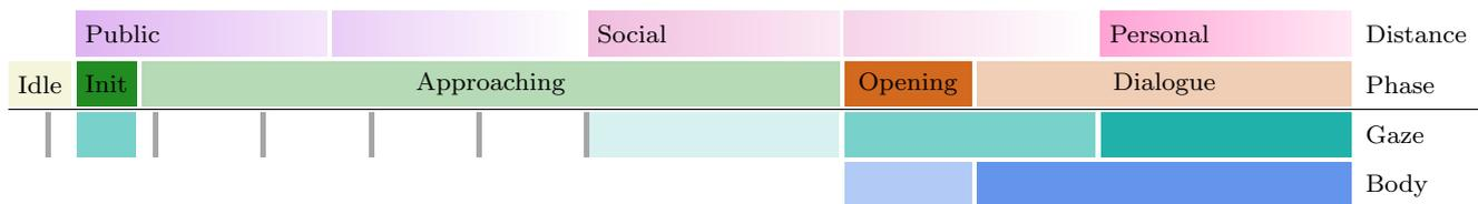
Fig. 3: Schematic depiction of the integrated attentive behaviour leading into a dialogue with a social robot. In the top row, the distance class between robot and human according to [20] is given. The second row describes the current phase or signal of the encounter (cf. Fig. 2). The bottom rows describe robot behaviour, i.e. rising attention towards the human with gaze (shades of cyan) interrupted by random gazes (grey) as well as via body orientation (shades of blue).
