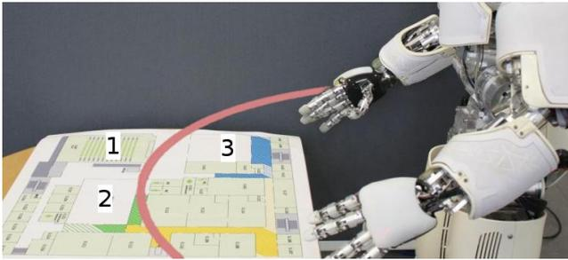
Fig. 7: Interactive area with a floor plan in front of the robot. A red line delimits the robot’s reaching space. Numbers 1-3 denote the locations that should be asked for in the study.
